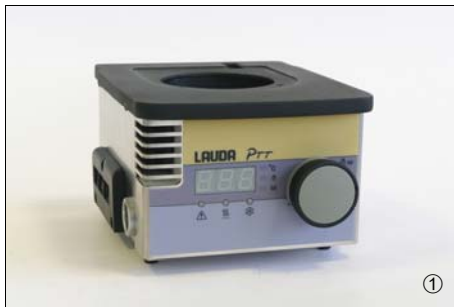
PTT Thermostating Unit
